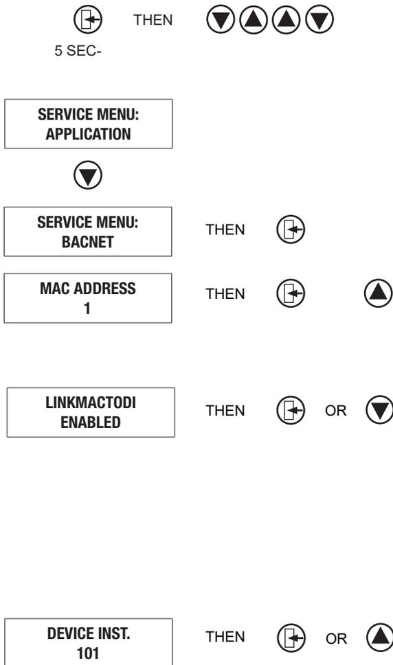
Hold down the **Menu** button on the LCD Thermostat for **5 seconds** until prompted for a passcode; use **▲** and **▼** to enter the passcode; **DOWN, UP, UP, DOWN**.
