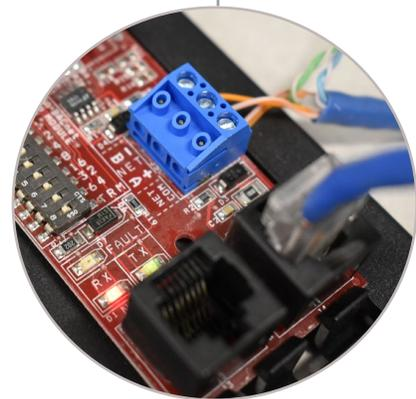
**NOTE:** BACnet terminal block and plug-and-play wiring can be used interchangeably.
